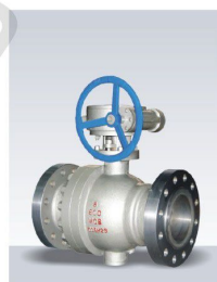
国标固定球阀 GB Fixed Ball Valve 公称通径: DN50~200mm Nominal diameter: DN50~200mm 公称压力: PN1.6~10.0MPa Nominal Pressure: PN1.6~10.0MPa 适用温度: -26℃~425℃ Applicable temperature: -26℃~425℃ 适用介质: 水、蒸汽、油品 Applicable medium: Water, steam, oil
