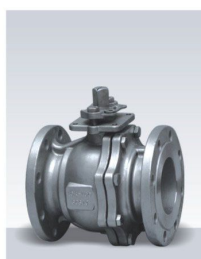
日标浮动球阀 JIS Floating Ball Valve 公称通径: DN1/2"~8" Nominal diameter: DN1/2"~8" 公称压力: PN150~600Lb Nominal Pressure: PN150~600Lb 适用温度: -26℃~425℃ Applicable temperature: -26℃~425℃ 适用介质: 水、蒸汽、油品、酸类 Applicable medium: Water, steam, oil, acid
