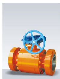
轨道球阀 Track Ball Valve 公称通径: DN1"~28" Nominal diameter: DN1"~28" 公称压力: PN150~1500Lb Nominal Pressure: PN150~1500Lb 适用温度: -26℃~600℃ Applicable temperature: -26℃~600℃ 适用介质: 水、油、天然气 Applicable medium: Water, oil, natural gas
