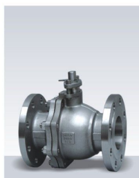
国标浮动球阀 GB Floating Ball Valve 公称通径: DN50~200mm Nominal diameter: DN50~200mm 公称压力: PN0.6~16MPa Nominal Pressure: PN0.6~16MPa 适用温度: -26℃~425℃ Applicable temperature: -26℃~425℃ 适用介质: 水、蒸汽、油品、酸类 Applicable medium: Water, steam, oil, acid
