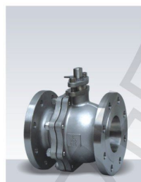
国标浮动球阀 GB Floating Ball Valve 公称通径: DN50~200mm Nominal diameter: DN50~200mm 公称压力: PN0.6~16MPa Nominal Pressure: PN0.6~16MPa 适用温度: -26℃~425℃ Applicable temperature: -26℃~425℃ 适用介质: 水、蒸汽、油品、酸类 Applicable medium: Water, steam, oil, acid
